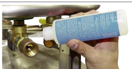
Oxygen Safe Valve Leak Check
