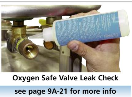
Oxygen Safe Valve Leak Check
