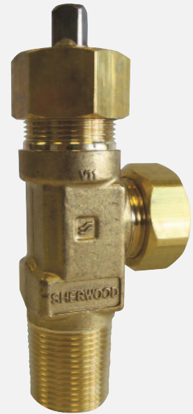
CGA 660 / 820 , CL-1 Thread, 158° Fuse-Metal Pressure Relief
