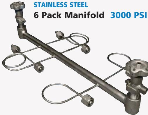
Constructed of 304 Stainless Steel and 3/4 inch NPT stainless valves and connectors, this manifold allows you to connect 6 cylinders at once for high volume hydrogen service applications.
