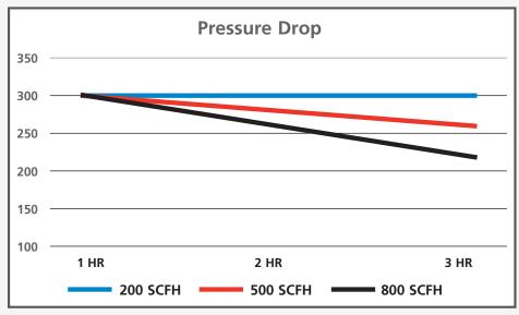
A liquid cylinder converting liquid into gas uses the vaporizer built into the liquid cylinder also known as the vaporizing coil and pressure building coil. The regulator is hooked up to the gas outlet. The pressure and flow rate drops when the demand exceeds the output capability of the vaporizing coil.
