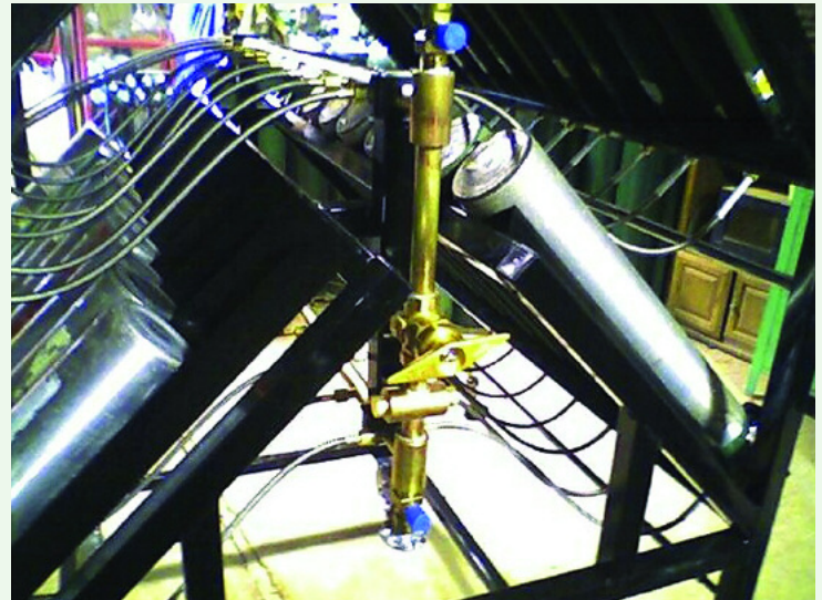
Isolation Master Valve for Filling Top and Bottom Rack Independently
