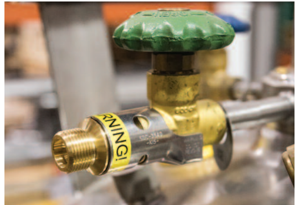
TPG restraints can only be removed by sawing off
