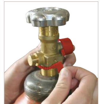
Breaking tamper evident seal – removing dust cover
