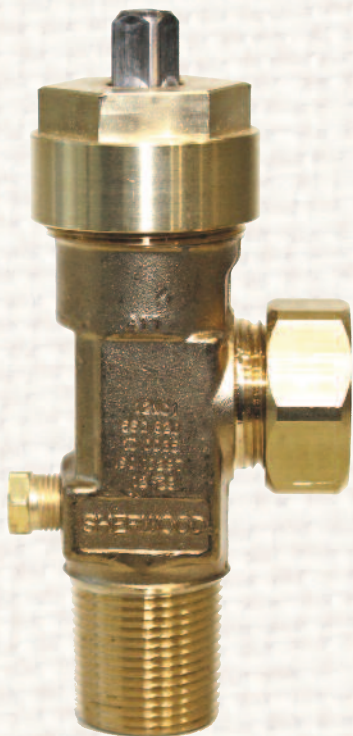
CGA 660 / 820 , CL-1 Thread, 158° Fuse-Metal Pressure Relief Part # SHW-1210AX1-CL1
