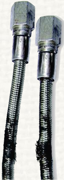
The braid on this hose was chemically attacked by an improper mixture of leak check solution.
