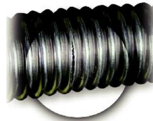
Circumferential cracks on the convolution are typically caused by high velocity flow rates
